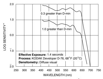
\*Sensitivity = reciprocal of exposure (ergs/cm<sup>2</sup>) required F002\_0511AC to produce specified density
