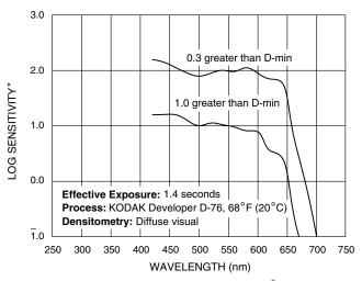
$\begin{tabular}{ll} *Sensitivity = reciprocal of exposure (ergs/cm^2) required \\ F002\_0523AC & to produce specified density \\ \end{tabular}$
