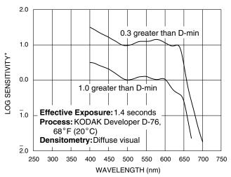
\*Sensitivity = reciprocal of exposure (ergs/cm2) required to produce specified density
